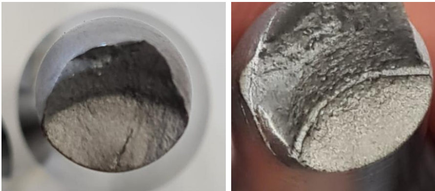
a) Core specimen failed due to large defect
