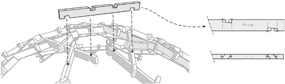
Figure 11. Detailing applied in the RFD with reinforcing screws and timber grain direction
