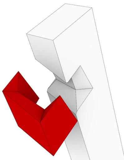
*Figure 13. Boolean intersection to create detailing with cutting shape (in red) and resulting detail*
