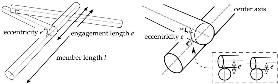
Figure 2. Parameters in a single-unit eccentric RF and eccentricity with its relation to member depth
