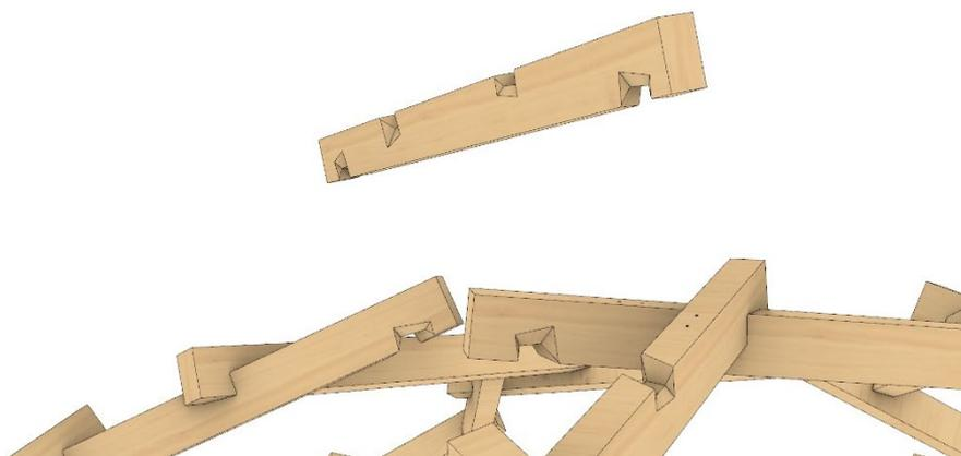
*Figure 12. Improved detailing by scaling the connecting planes of the notches*
