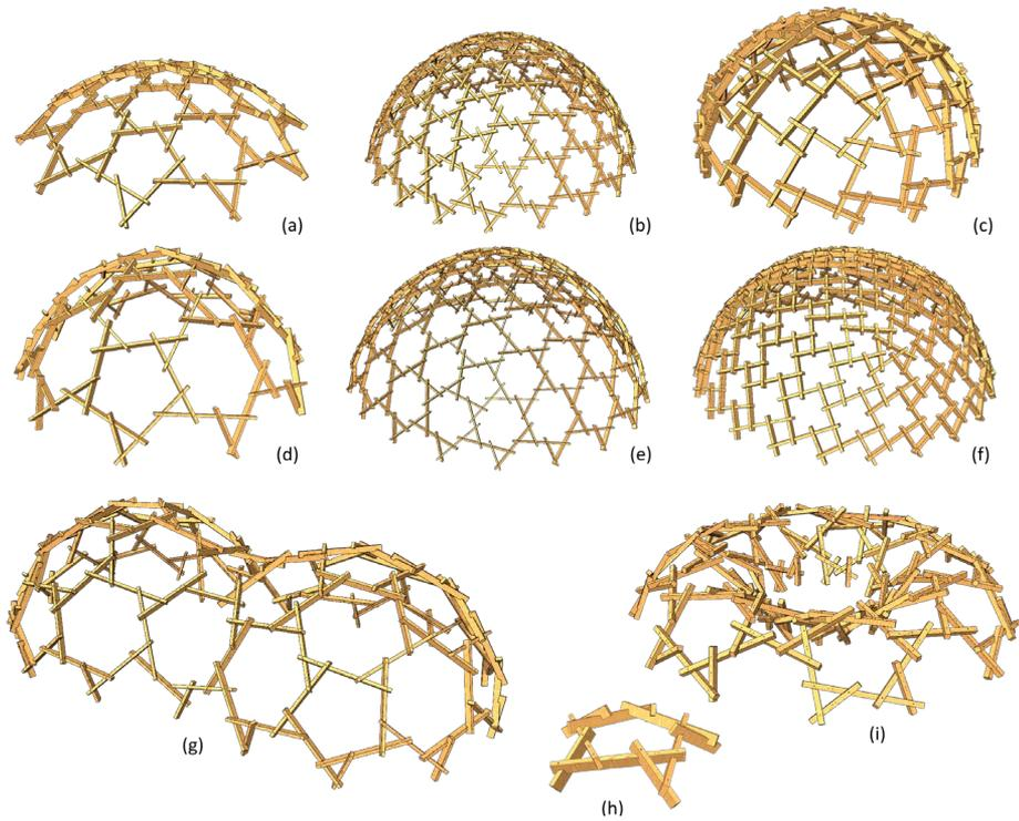
Figure 26. Nine possible RFD results covering the same span based on geodesic icosahedra (a, b, d, e), cubes (c, f)
