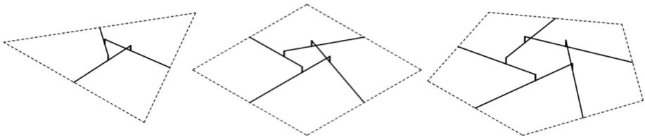
Figure 4. Three single RF units with elevated intersection points
