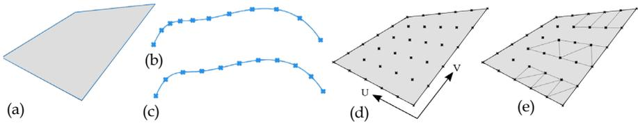
Figure 5. NURBS surface (a), by means of parametric curvature (b) or equal point distance (c) subdivided in UV direction by points (d), after which these can be panelized (e) by geometrical rules
