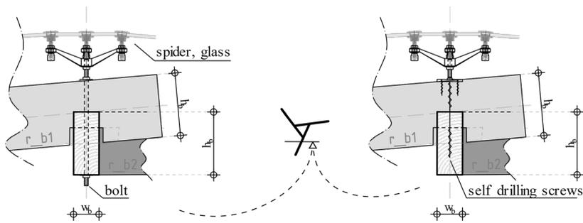
Figure 27. Concepts for roofing on an RF structure
