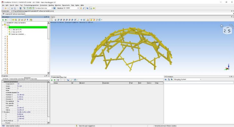
Figure 19. A direct RF import from the RFD in Grasshopper to Cambium. Cambium is the driving CAM software of Hundegger machines. Timber beams can directly be machined from this file
