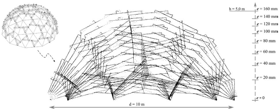
Figure 10. The influence of different chosen eccentricity values ( $e$ ) on the structural height of an RF while using the same scaling factor (scaling factor see figure 3.3)
