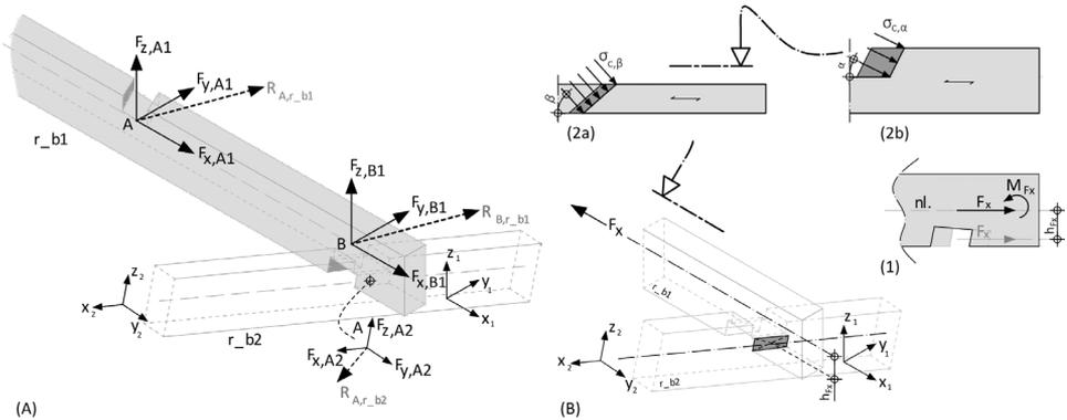
Figure 15. Force distribution/identification from one member to another, stress at angle to the grain
