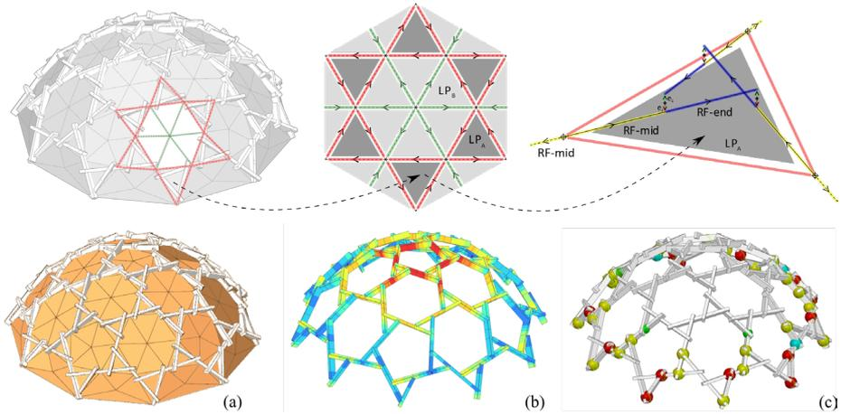
Figure 16. Structure of FE model: Load panels (a), illustrative FE model with bending moment  $M_{yy}$  (b), UCs > 1 according to EN1995 (Eurocode 5) showing timber failure in the RFD (c)
