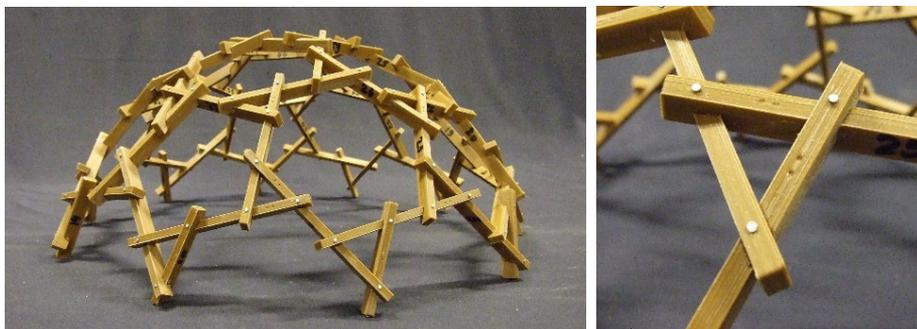
Figure 22. 3D printed 1:20 scale model using the same design as displayed in figure 10 with  $e = 100$  mm. The two dots on each beam indicate the highest point of each beam allowing ease of construction.
