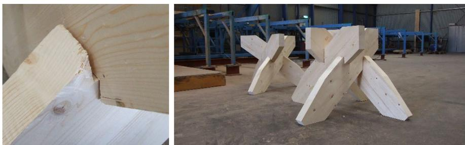
Figure 21. Full scale model made with CAM and Hundegger machine to test the feasibility of RF detailing
