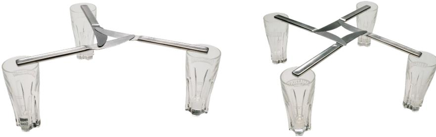
*Figure 1. The structural principle of a three- and four-member single unit reciprocal frame*
