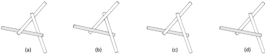
Figure 8. Four possible three-member unit styles. Unit style (a) and (b) can be structurally stable from itself by utilizing friction or using notching between the members
