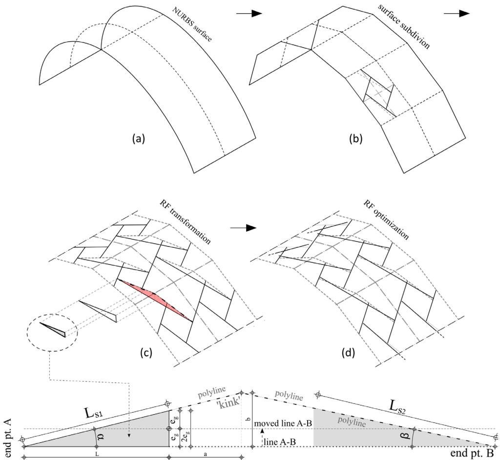
Figure 7. Basic geometrical design procedure that has been applied in the RFD
