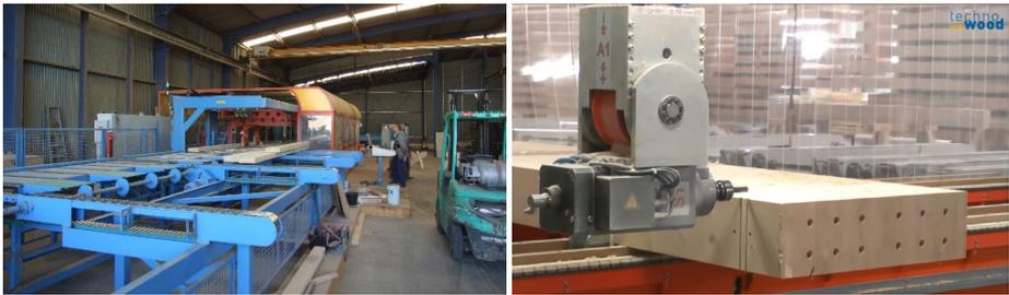
Figure 17. Hundegger machine (left) and timber milling in a Technowood machine (right)
