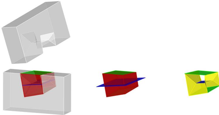
*Figure 14. The Boolean intersection geometry creation method with a red/green cube as geometrical basis with resulting geometry on the right in blue and yellow*
