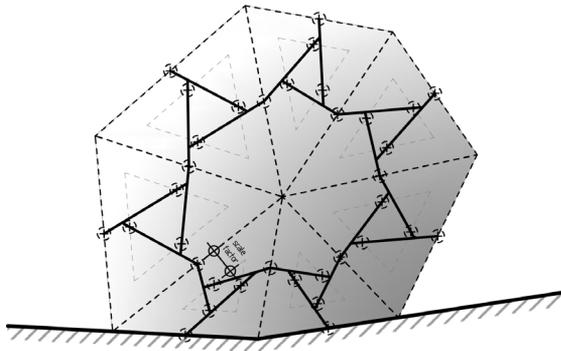
Figure 6. Center to center method applied to a faced Brep or mesh
