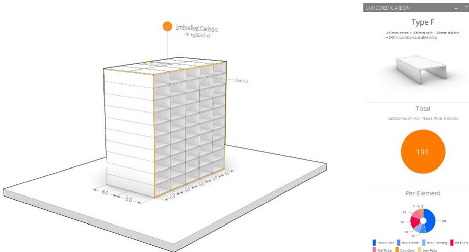
Figure 5. Exploring structural embodied carbon of building (© Arup)
