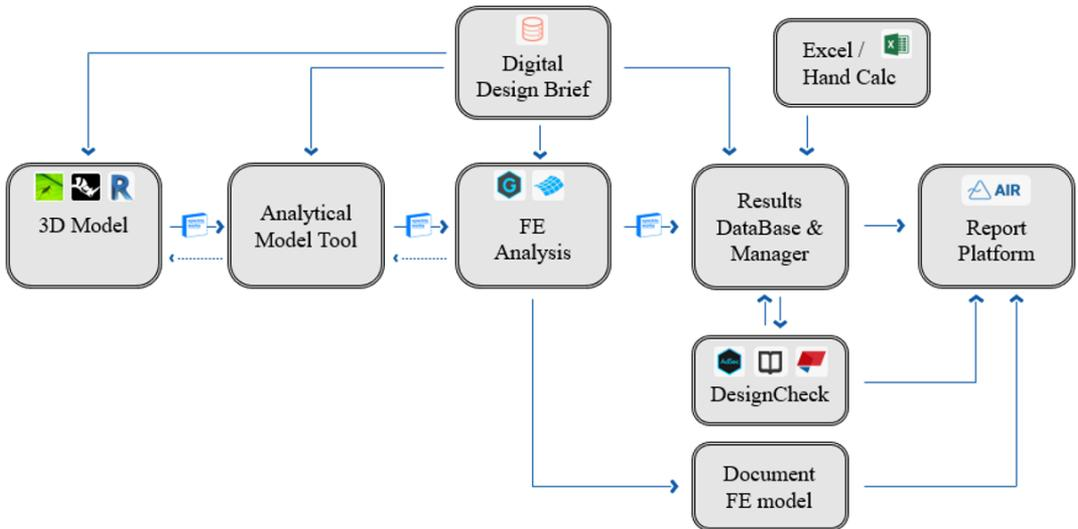
Figure 14. Overall structural design workflow (©Arup)
