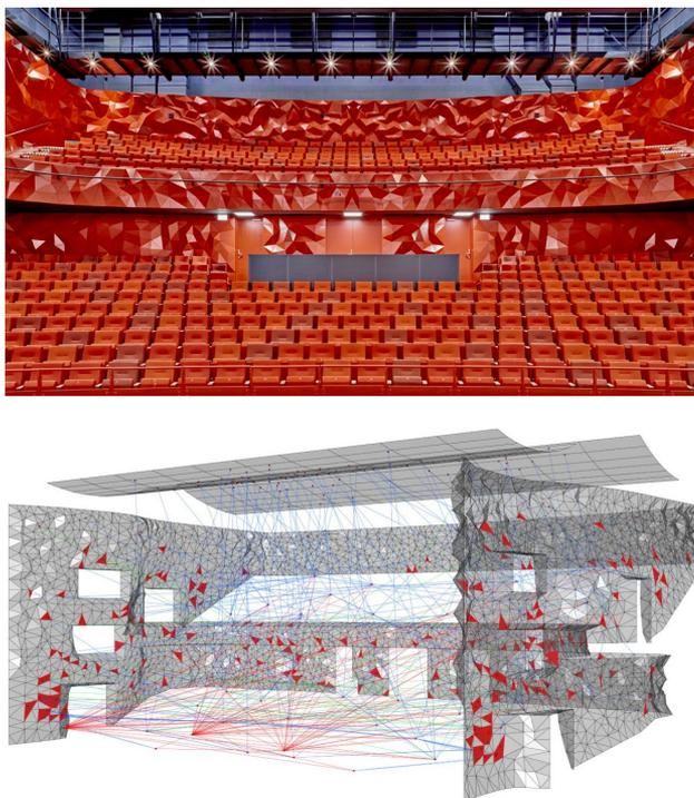
Figure 17. Parametric design and optimisation of Theater Zuidplein Rotterdam (Left: © Pim Top; right: © Arup)
