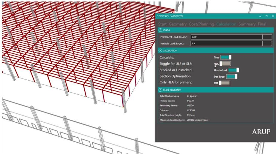
Figure 13. Automated steel platform design (©Arup)
