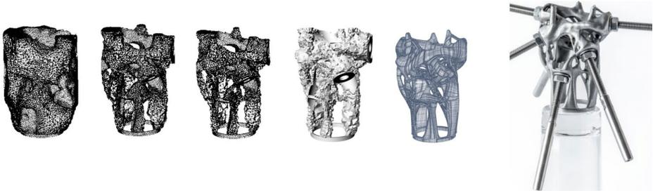
Figure 10. Topology optimisation process of the Arup AM metal node (©Arup)
