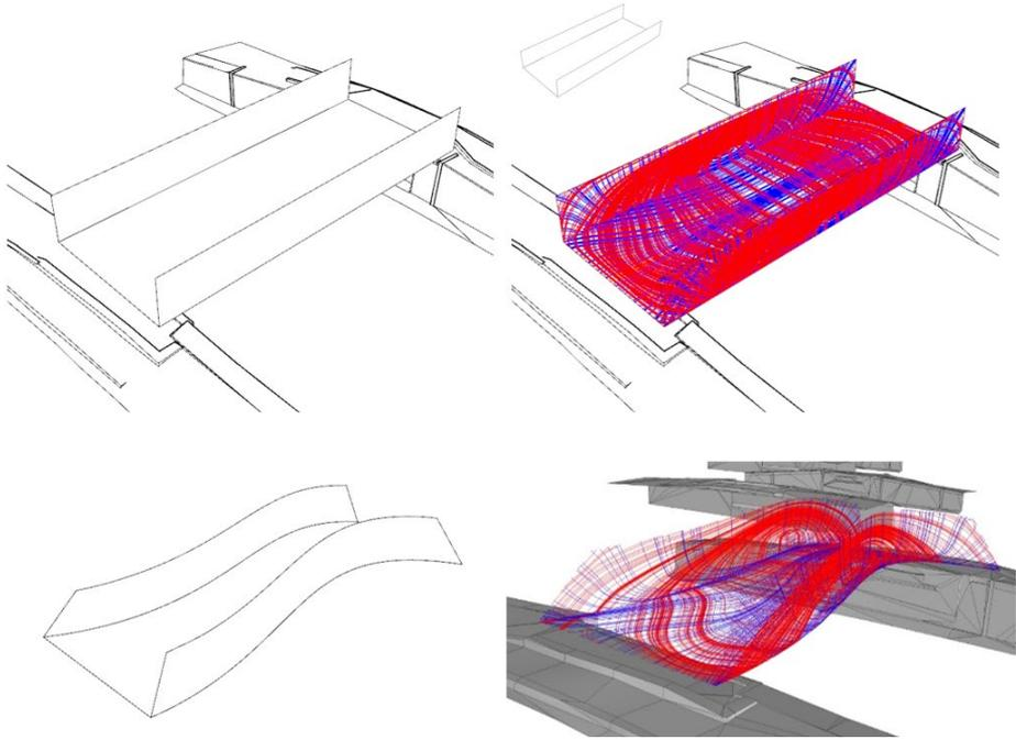
*Figure 15. Structural form-finding with the stress lines of MX3D bridge (©Arup)*
