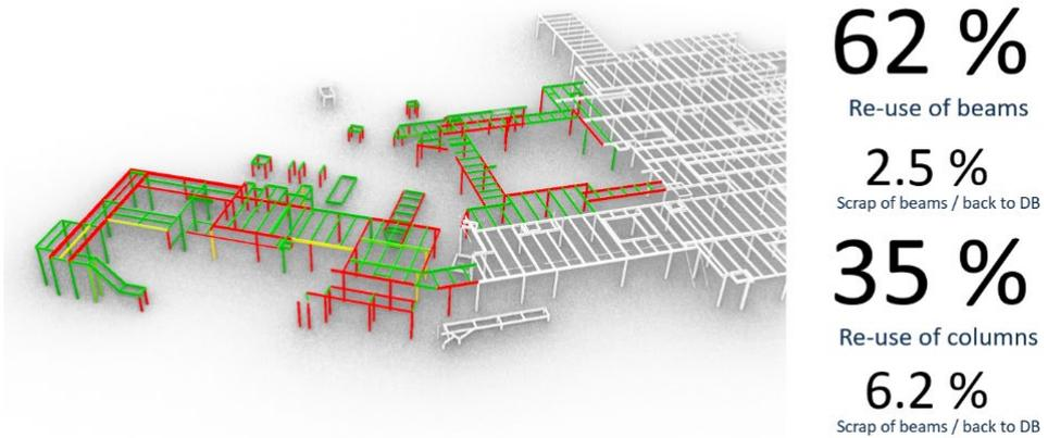
Figure 6. Designing steel structure with reusable steel members (© Arup)
