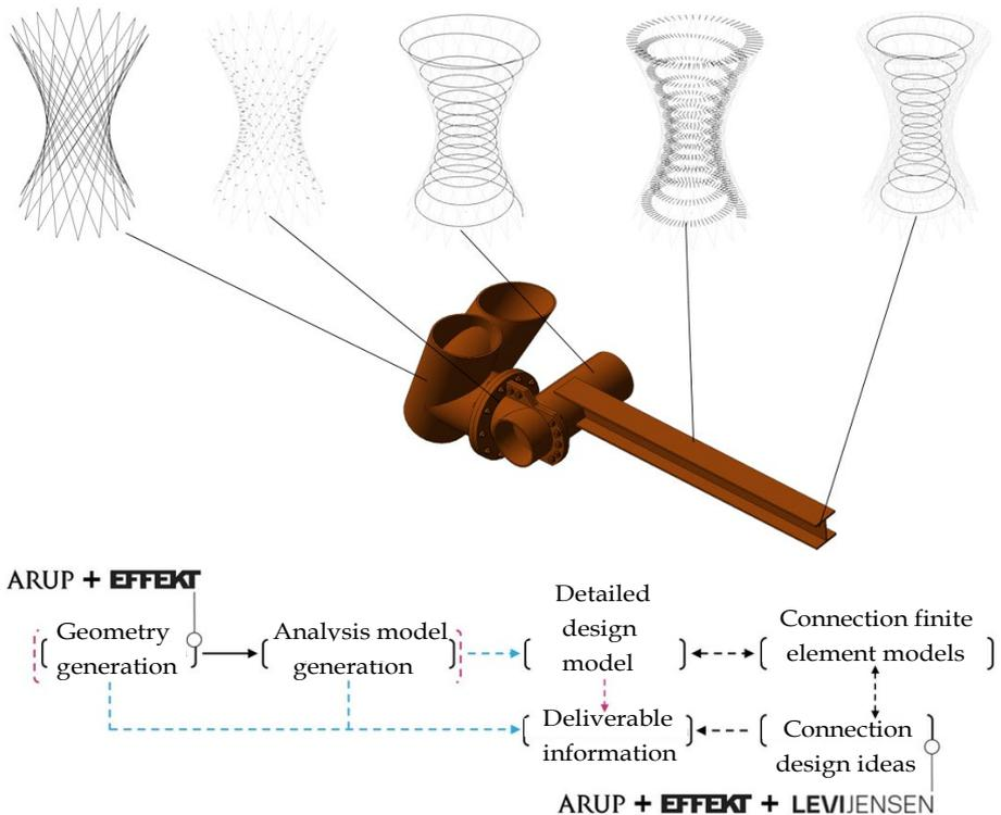
Figure 4. Parametric workflow developed for Camp Adventure Tower (© Arup)
