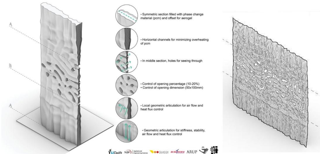
Figure 21. DoubleFace 2.0 Solar Wall 3D diagram (©TU Delft)
