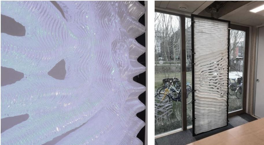
Figure 22. DoubleFace 2.0 Solar Wall full-scale mock-up (©TU Delft)
