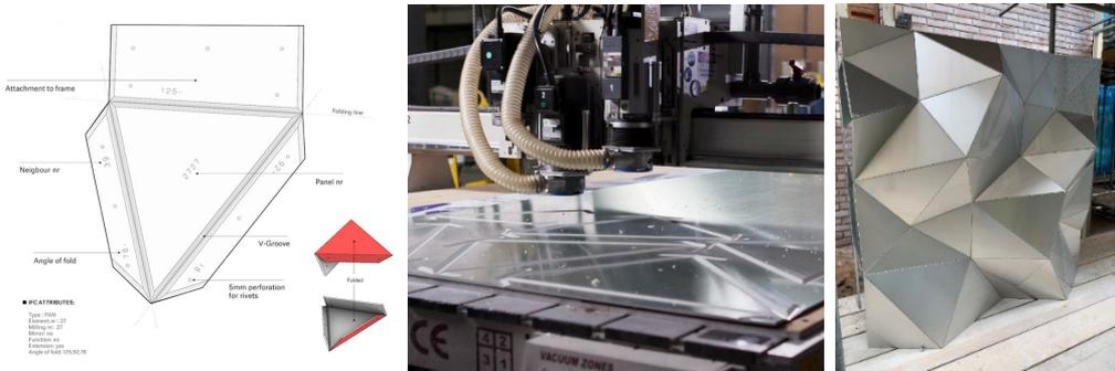
Figure 18. Digital fabrication with CNC and the mock-up (Left and middle: © StudioRAP & Aldowa; right: © Arup)
