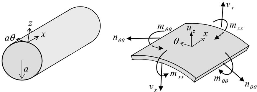
Figure 2. Circular cylindrical shell; Stress resultants; Sign convention
