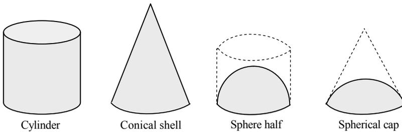
Figure 1. Four different shells of revolution
