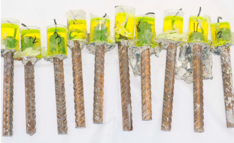
Figure 11. Surface condition of steel reinforcement in BFS specimens after 6 months of exposure
