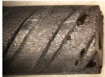
b) Corrosion pits in PC-2
