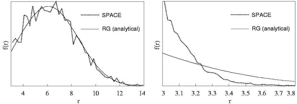
Figure 2. Deviations between predictions on nearest neighbor density distributions,  $f(r)$ , at 1% (left) and 30% (right) by volume of 3 mm particles obtained by a random generator (RSA system), and by a concurrent algorithm based (SPACE) computer simulation system. For the RSA simulation the theoretical Poisson estimate is used. Already at a volume percentage of 30, the deviations in aggregate or cement grain distributions would be dramatic between RSA and DEM.
