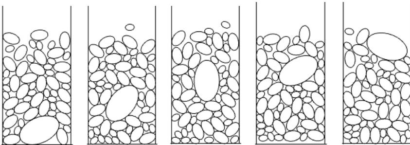
Figure 1. Traditional Brazil nut concept: mixture of non-spherical particles of various sizes is activated by vibration at the bottom of the container. Sequence is displayed of 2D simulations by DEM system HADES during the size segregation process (stills of video).
