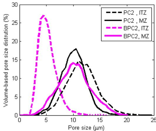
Figure 7. Pore size distribution functions for plain (PC2) and blended Portland cement (BPC2) pertaining to the ITZ (dashed line) and to the middle zone (MZ) between the ITZs (continuous line).
