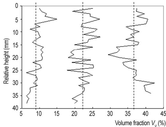
Figure 3. Gradient structures in volume fraction ( $V_v$ ) of coarse aggregate (dashed lines indicate averages in different concrete mixtures). Top of specimen is at the bottom of the scale.
