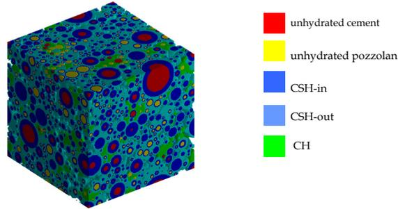
Figure 6. Visualization of the hydrating paste. Each unhydrated multi-phase core is represented by a sphere whose volume equals the total volume of the phases. (This figure is in colour at [www.heronjournal.nl](http://www.heronjournal.nl))
