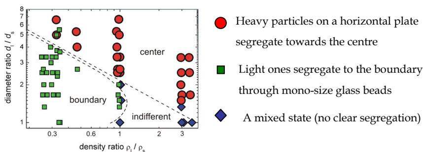
Figure 4. Phase space for particle properties. Each symbol represents one experiment. Shaker amplitude of an horizontal disk is 1.91 cm and frequency 1.67 Hz. Mechanisms were also depending on the area percentage of filling the disk with the glass beads (segregation was not observed at lower values).
