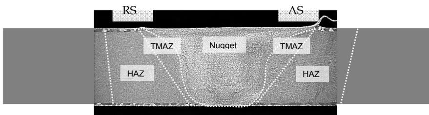
Figure 1: Zones of the friction stir weld – weld nugget, thermomechanically affected zone (TMAZ), and heat affected zone (HAZ). The advancing side (AS) and the retreating side (RS) of the weld are also indicated.
