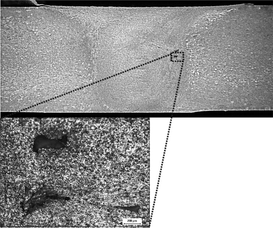
Figure 2: Friction stir weld with running void in aluminium alloy AA6061-T6
