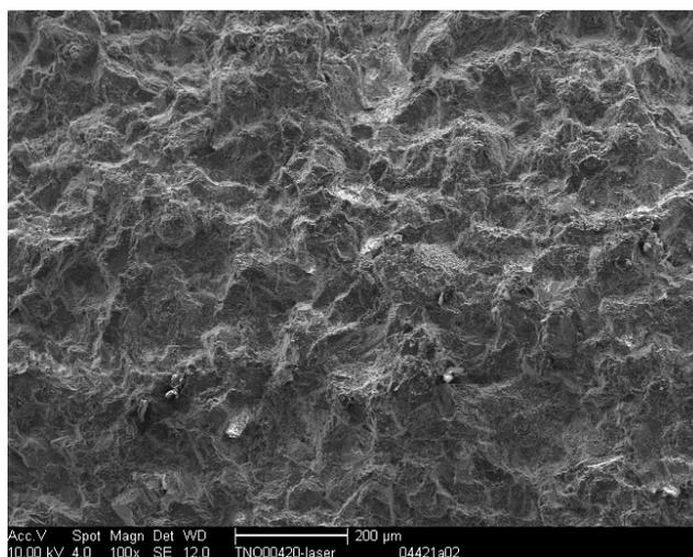
*Figure 12: SEM microphotograph of the surface of Obernkirchen sandstone from test panel A cleaned by dry microblasting followed by laser (sample TNO 00420)*
