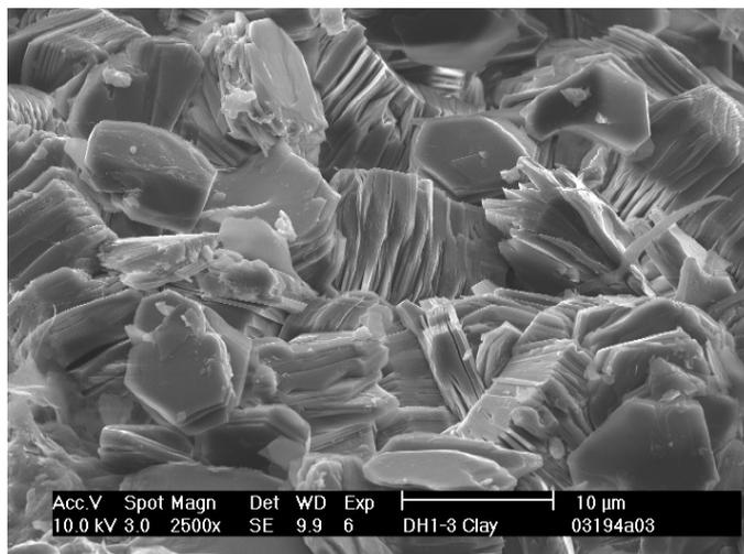
Figure 2: SEM microphotograph showing the pore filling of Obernkirchen sandstone by kaolinite (sample TNO 00420)
