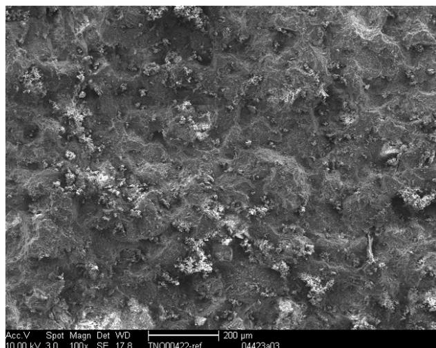
*Figure 11: SEM microphotograph of the surface of non-cleaned Obernkirchen sandstone from test panel A (sample TNO 00422)*
