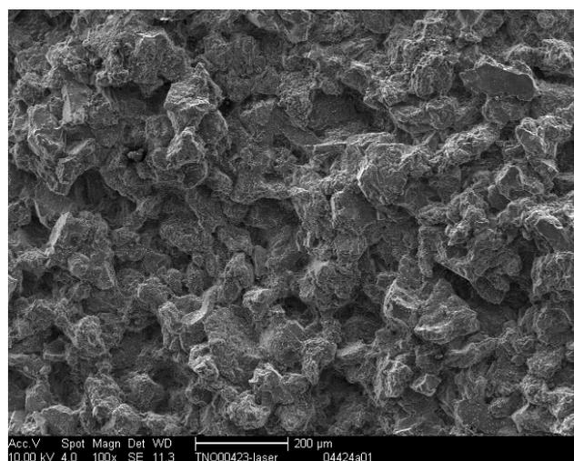
*Figure 14: SEM microphotograph of the surface of Obernkirchen sandstone from test panel A cleaned by laser at maximum intensity (sample TNO 00423)*
