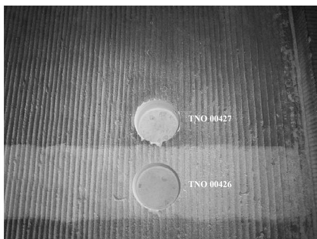
*Figure 8: Overview of samples for microscopic evaluation obtained from test panel C*
