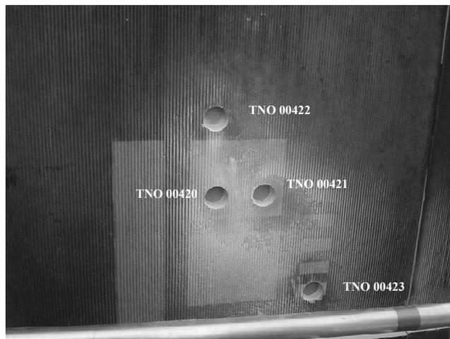
*Figure 6: Overview of samples for microscopic evaluation obtained from test panel A*
