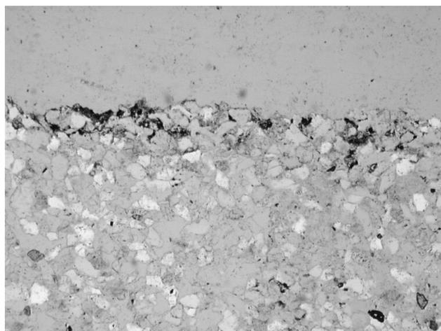
*Figure 9: Microphotograph showing the nature of the thin black weathering layer on non-cleaned Obernkirchen sandstone (sample TNO 00422, plane polarized light, view 2.7 x 1.8 mm)*
