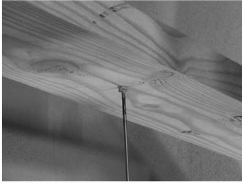
Figure 4: Transducer attached to specimen
