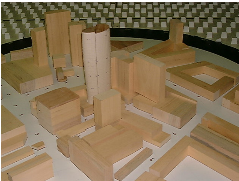
Figure A1: Building with changing plan in height; upper floors are trapezium shaped, with rounded corners
