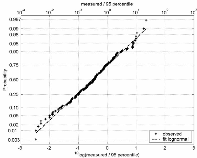
Figure 3: Frequency distribution of  $\log g_{\text{high}}$  the logarithm of the ratio of measured values and the experts' 95-percentiles. The frequency distribution is plotted on normal probability paper.
