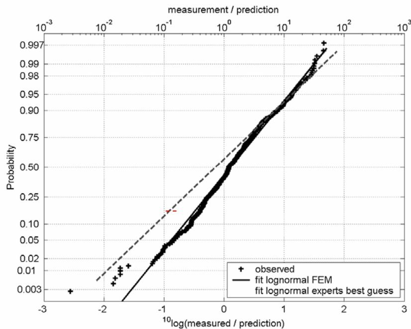
Figure 5: Frequency distribution of  $\log g$ , the logarithm of the ratio of measured values and the FEM-predictions. The frequency distribution is plotted on normal probability paper. For reference the distribution fitted to the experts’ best guesses is also shown (dashed line).
