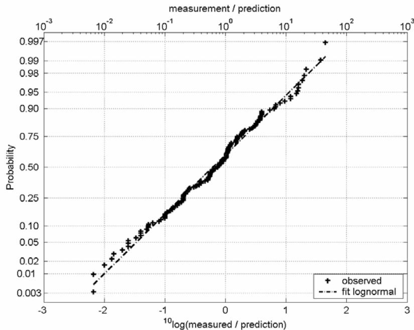
Figure 2: Frequency distribution of  $\log g$ , the logarithm of the ratio of measured values and the experts' best guesses. The frequency distribution is plotted on normal probability paper.
