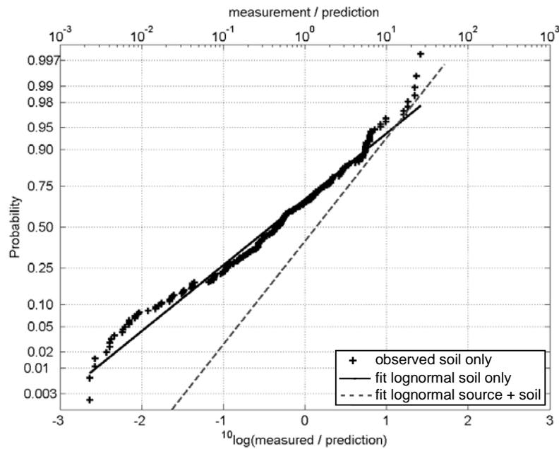
Figure 6: Frequency distribution of  $\log g$ , the logarithm of the ratio of measured values and the FEM-predictions for the soil subsystem only. The frequency distribution is plotted on normal probability paper. For reference the distribution fitted to the FEM-predictions for the system 'source+soil' is also shown (dashed line).
