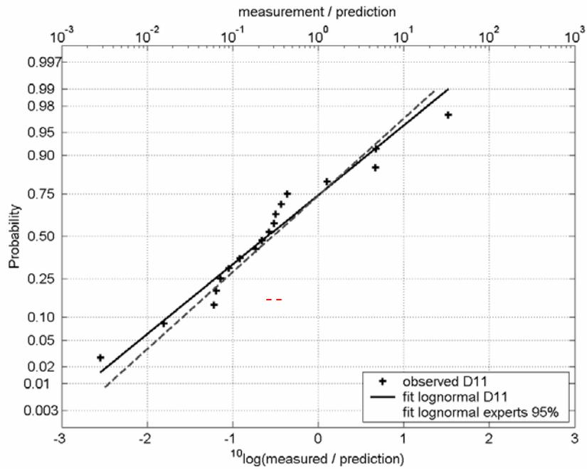
Figure 4: Frequency distribution of  $\log g$ , the logarithm of the ratio of measured values and the D11 predictions. The frequency distribution is plotted on normal probability paper. For reference the distribution fitted to the experts' 95-percentiles is also shown (dashed line).
