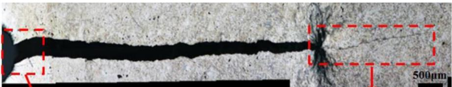
Figure 12: Crack flank before and after an overload, optical microscope image of 304L stainless steel. Image from [59]. Box left-hand side: initiation of the crack from a notch. Box right-hand side: crack flank developed after the overload.
