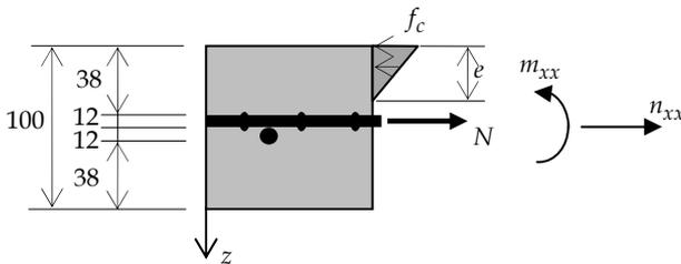
Figure 8. Reinforcement in the middle of the shell thickness
