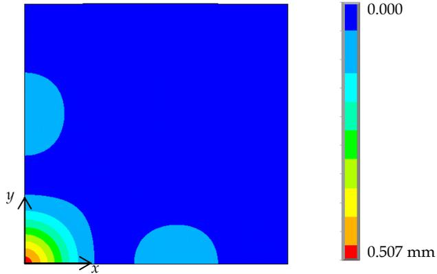
Figure 4. Deformation of the hyper shell (displacement length)
