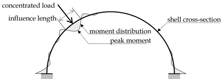
Figure 1. Moment distribution in a shell cross-section due to a concentrated load
