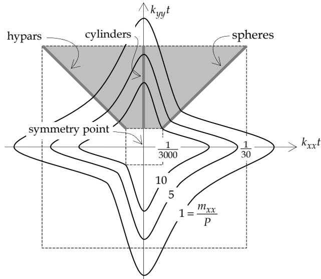
Figure 7. Possible contour lines of  $\frac{m_{xx}}{P}$
