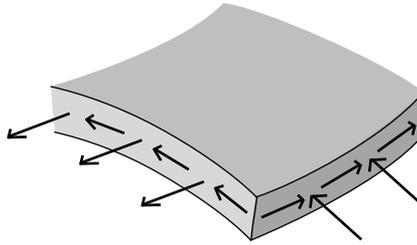
Figure 3. Corner of a shell with the edge support reactions
