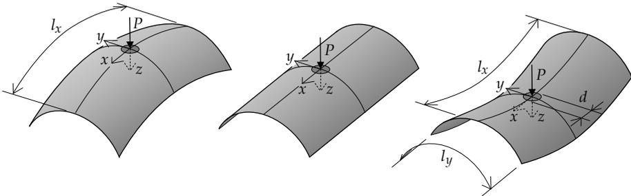
Figure 2. Shell shapes with concentrated loads and coordinate systems
