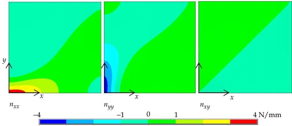
Figure 5. Membrane forces in the hyper shell
