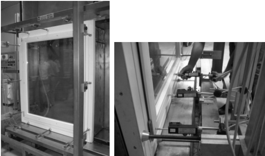
Figure 4. Test set up and placement of measurement devices according to EN 12211:2000 [2]
