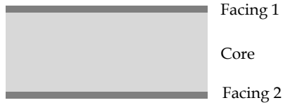
Figure 1. Composition of a typical sandwich element
