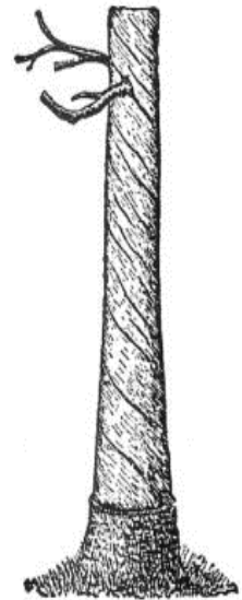
Figure 11. Spiral grain (Kollmann 1968)
