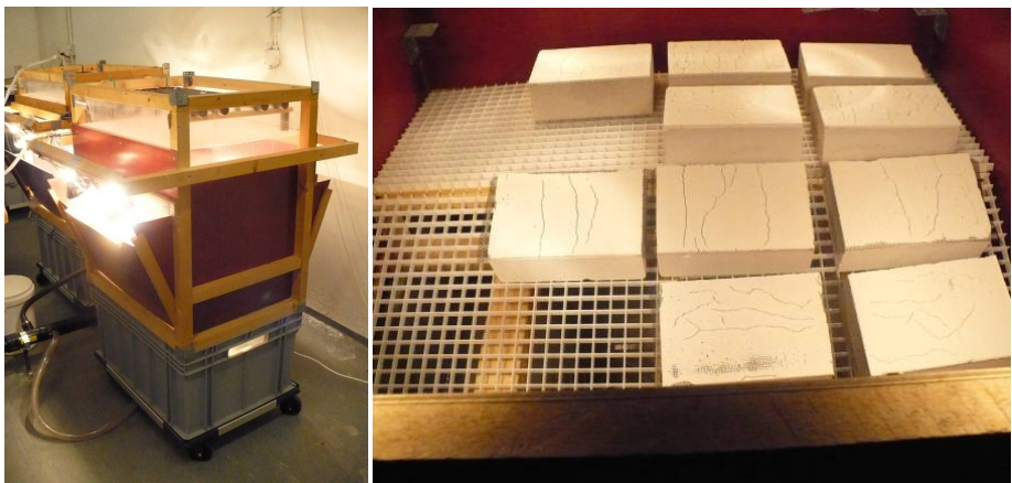
Figure 3. Artificial rain set-up (left) with the samples (right)
