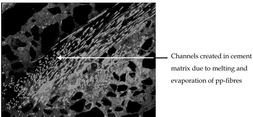
Figure 6: PFM-microphotograph taken at about  $20 \text{ mm}$  from spalled surface element, B, containing  $3 \text{ kg.m}^{-2}$  pp-fibres. View is  $2.7 \text{ mm} \times 1.8 \text{ mm}$ .
