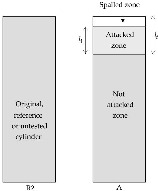
*Figure 9: Schematic diagram, not drawn to scale, showing the method by which the depth of attack was determined from the tested tunnel elements. R2 = reference, dummy or untested cylinder, A = one of the tested elements showing the various zones that were used in the analysis.*
