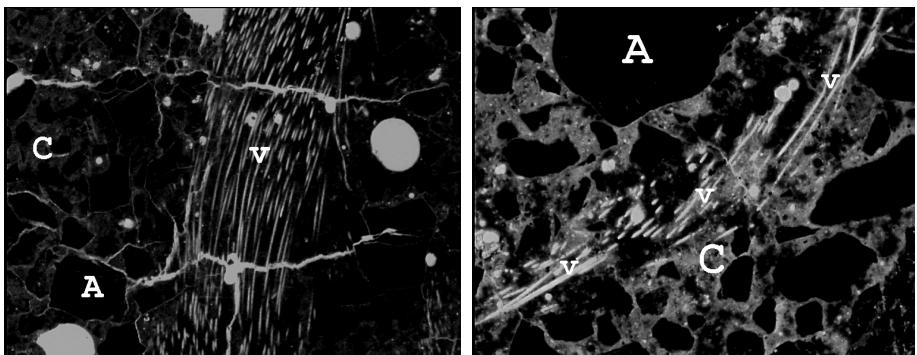
Figure 7: PFM-photomicrographs taken at about 20 mm from spalled surface of both elements showing development of channels and microcracks in cement paste. A = aggregate; C = cement paste matrix; v = pp-fibres.
