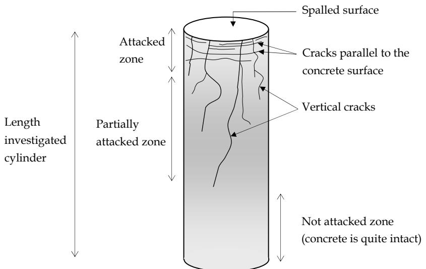
*Figure 8: Schematic representation of the microscopic features observed from PFM analysis of thin section specimens*
