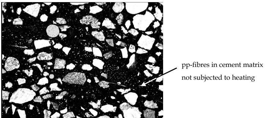
Figure 5: PFM-microphotograph of reference element, R2, containing  $2 \text{ kg.m}^{-2}$  pp-fibres showing distribution of pp-fibres in cement paste matrix. Concrete was not exposed to fire. View is  $2.7 \text{ mm} \times 1.8 \text{ mm}$ .
