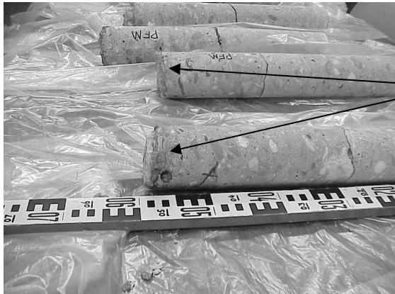
*Figure 2: Overview of some of the cores removed from the two concrete elements for the microscopic studies showing the spalled surfaces and colour changes caused by fire heating*
