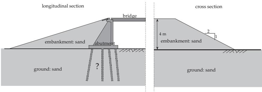
Figure 1. Example 1: Abutment foundation: situation sketch
