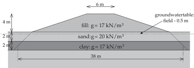
Figure 3. Embankment; geometry and specific weights
