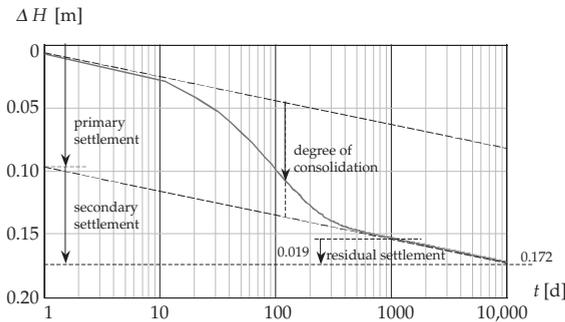
Figure 4. Embankment; settlement versus logarithmic time
