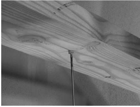
Figure 4: Transducer attached to specimen
