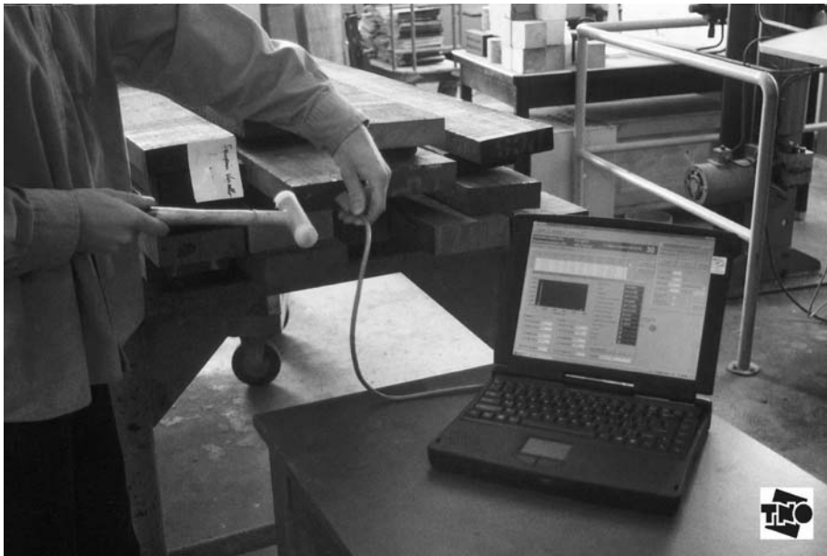
Figure 20: Lab prototype of the Mobile Timber Grader. Beams of different wood species and different sizes can be graded.
