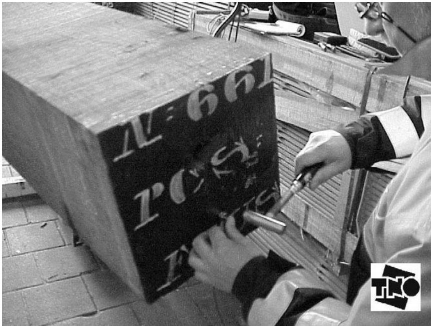
Figure 21. The Mobile Timber Grader makes it possible to machine grade beams of large sizes.
