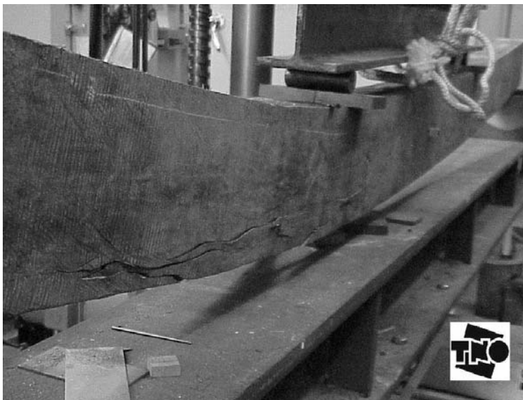
Figure 6: The static modulus of elasticity is calculated out of the deflections measured in a four-point bending test according to EN 408.
