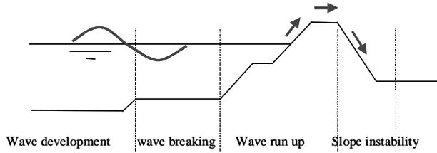
Figure 5: Dike failure mechanism: overtopping
