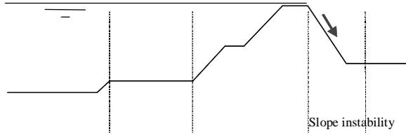
Figure 6: Dike failure mechanism: overflow
