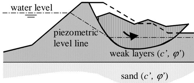
Figure A2: Dike failure mechanism: sliding of the inner slope
