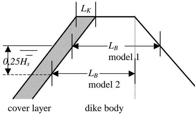
Figure A3: Dike failure mechanism: erosion of dike body
