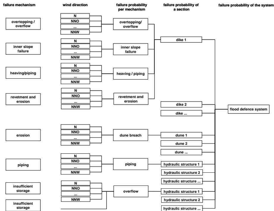
Figure 1: Flow chart for the failure of a flood defence system
