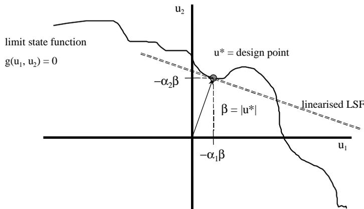
Figure 2: Two-dimensional illustration of  $u$ -space, limit state function and design point
