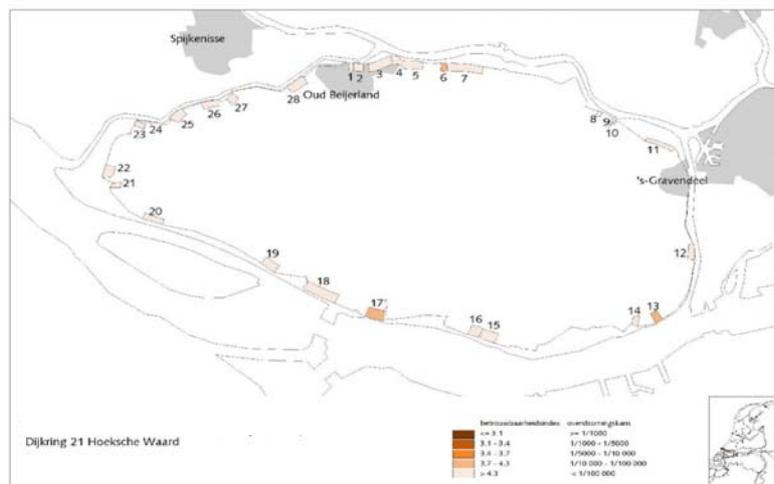
Figure 7: Overview of the flood defence system 'Hoeksche Waard'. The numbers refer to the section which are analysed
