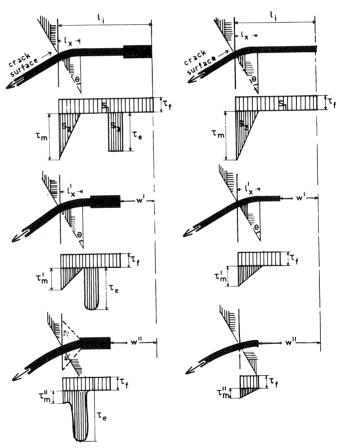
Fig. 20. Geometrical changes occurring during fibre pull-out and the assumed interfacial shear stress distributions.
