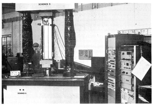
Fig. 4. Testing arrangement for the direct tension experiments.
