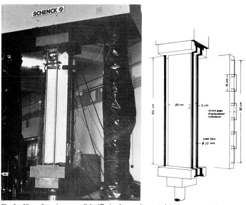
Fig. 5. View of specimen, parallel stiffening bars and mounted strain gauge transducers and travelling microscope.
