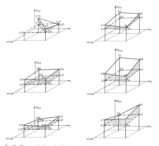
Fig. 12. Fibre contribution to the ultimate tensile strength as revealed in the direct tensile test (at the left) and the Brazilian splitting test (at the right) and shown as a function of the water to cement ratio and the fineness modulus. From top to bottom: straight, hooked and paddled fibres, respectively. Results in N/mm<sup>2</sup>.
