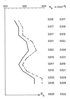
Fig. A2. Variation of the number of fibres per unit of area along the specimen axis. Comparison of two quantitative image analysis techniques. The solutions are based on the partially planar-oriented structural model for the fibre dispersion in the specimen. The feature counting was executed over the entire cross section, whereas the intersection counting omitted the most severely disturbed areas near the casting (viz. e.g. Stroeven [1979]). The presented examples are two extreme cases.
