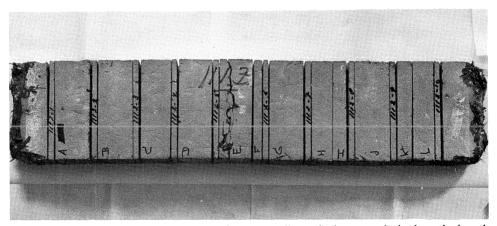
Fig. 6. Arrangement of the slices applied for X-ray radiography image analysis along the length of a specimen.
