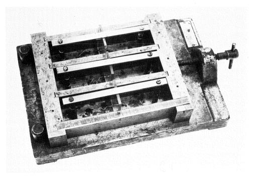
Fig. 3. Mould for the pull-out specimens prior to filling up with the mortar.
