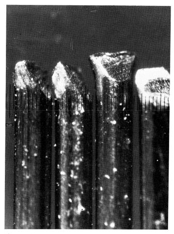
Fig. 8. Magnification of the straight fibres used in the investigations, revealing the screwdriver fibre ends.
