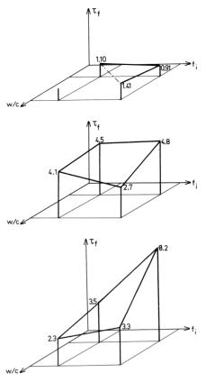
Fig. 13. Dynamic friction resistance,  $\tau_f$ , as calculated from eq. (5), shown as a function of the water to cement ratio and the fineness modulus. From top to bottom: the straight, the hooked and the paddled fibres, respectively. Results in N/mm<sup>2</sup>.
