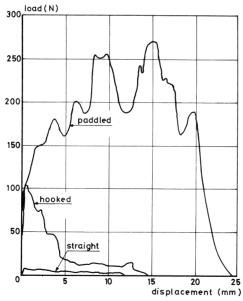
Fig. 7. Typical load-displacement curves for the three types of fibres encompassed in the pullout experiments.
