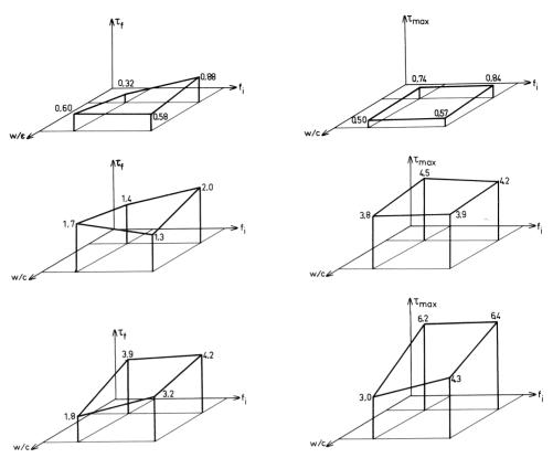
Fig. 9. Dynamic friction resistance,  $t_f$ , and maximum shear strength,  $t_{max}$ , both as a function of fibre type, water to cement ratio and fineness modulus. From top to bottom: straight, hooked and paddled fibres, respectively. Results in N/mm<sup>2</sup>.
