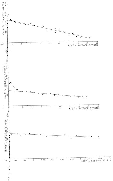
Fig. 10. Typical examples of approximated stress-strain diagrams, from top to bottom representing FRC specimens containing straight, hooked and paddled fibres, respectively.
