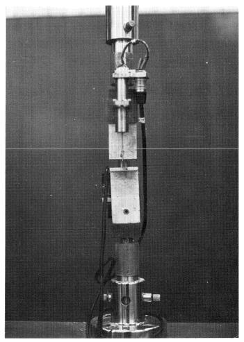
Fig. 2. Detail of the mortar specimen in the Instron testing machine at termination of the pullout test.
