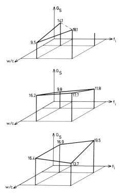
Fig. 16. Specific toughness results for the three fibre types FRC specimens shown as a function of the water to cement ratio and the fineness modulus. From top to bottom: straight, hooked and paddled fibres, respectively. Results in N/mm.
