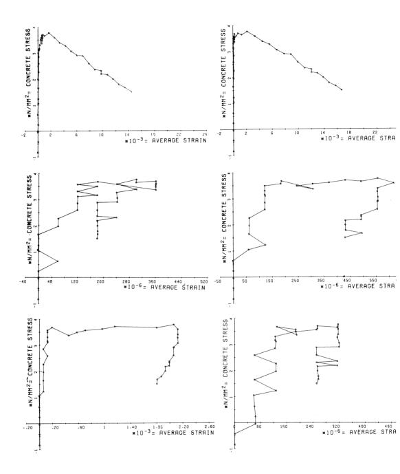
Fig. 19. Examples of stress-strain curves of neighbouring regions (transducers 7 to 12) of a FRC specimen containing hooked fibres. Cracking in the weakest region (at the top) is accompanied by micro- and sub-macrocracking up to various degrees in other regions. Crack initiation takes place at different percentages of ultimate in the different measuring sections. Note that the zero stress level is situated at -0.56 N/mm<sup>2</sup>.
