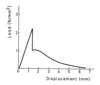
Fig. 15. Typical stress-strain curve for a FRC specimen in tension containing straight fibres.
