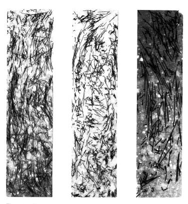
Fig. A1. X-ray radiographs of thin elements of FRC specimens containing the three applied commercial fibre types. From left to right: the straight, hooked and paddled fibres, respectively.
